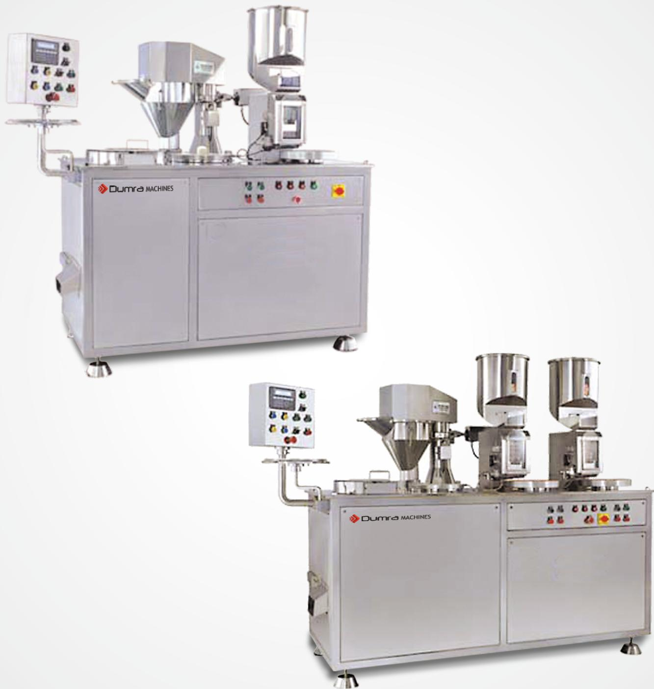
DUMRA semi automatic capsule filling machines are user friendly and are available in two models - Single Head and Double Head with advanced features. They are designed for precision manufacturing requirements of latest pharmaceutical procedures and also ensure cleanliness and product integrity. The machine provides a high degree of automation with higher levels of filling weight accuracy. These machines are suitable for filling capsule of all size with powder, pellets and granules.
